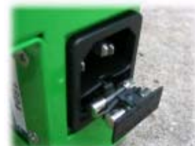
IEC power socket showing fuse draw open
